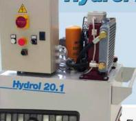
Hydrol 20.1 hydraulic unit, supplied with expansion setting control, has compact dimensions, for easy transport and movement on site. Torque value is regulated by an adjusting pressure setting on the hydraulic unit.
