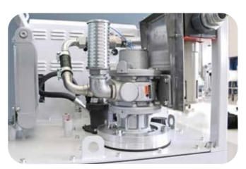
Hydraulic oil filter with mechanical indicator for hydraulic oil filter change warning.
