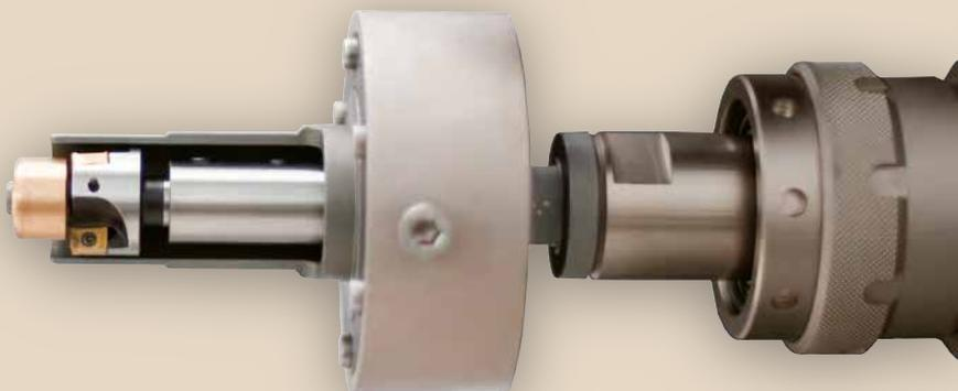
Quick connect tube end facer-holder complete with rotating distributor for lubrication
