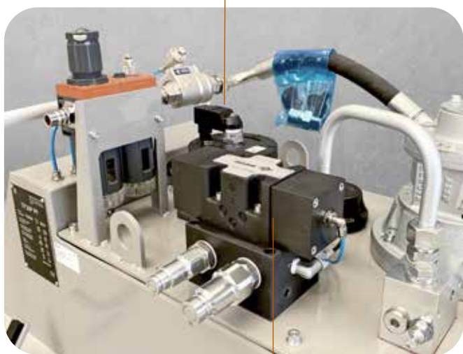
Pneumatic valves in manual / automated mode
