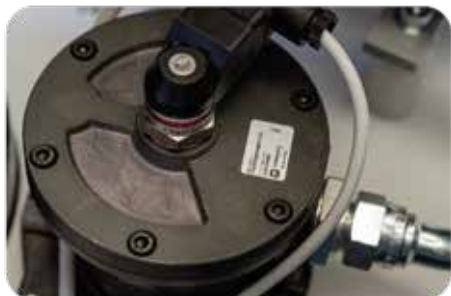
Hydraulic oil filter with electrical signalling for filters to be replaced
