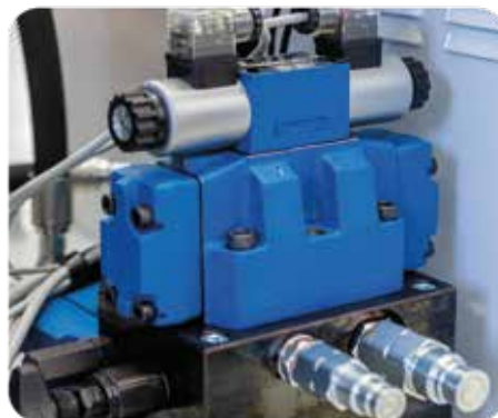
Electrovalves in automated / manual cycle (slow/fast) Hydraulic oil flow and pressure regulation
