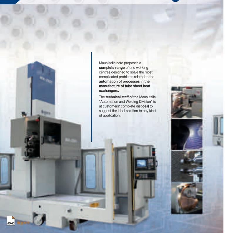
Cnc working centre with single axis fixed machine to expand and face the tube bundle tubes.
